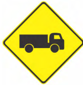
FIGURE 5.11 – TYPICAL W5-22 SIGN FACE (TfNSW)
